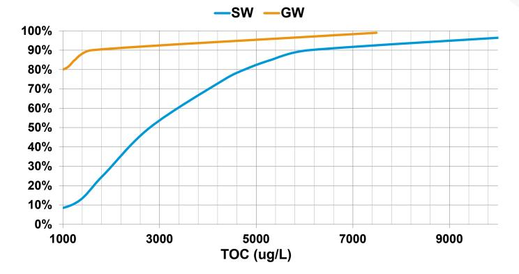
Although, as expected, TOC is much higher in SW systems than GW systems, nearly 10% of GW samples have TOC > 3000 ug/L, which could lead to measureable DBPs.
