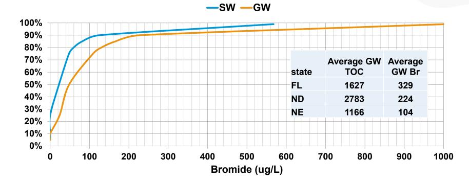
Br levels in GW systems are generally higher than SW, but won't have as big an effect on DBPs because of lower TOC levels. FL, ND, and NE all are likely to have Brominated HAA in GW systems.
